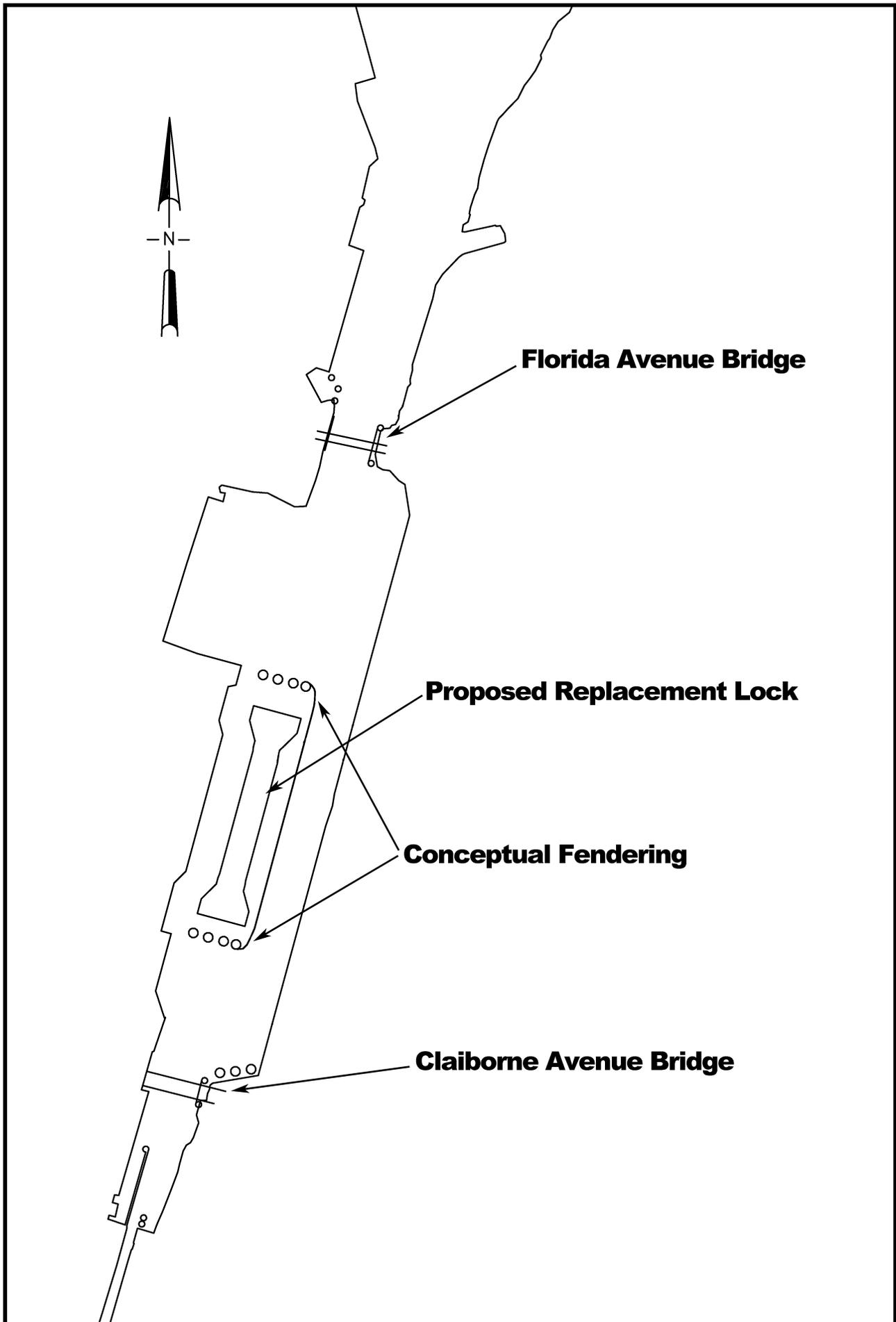
**Figure 5. Conceptual Fendering to tie into protection cells for the Float-in-Place Construction Alternative**
